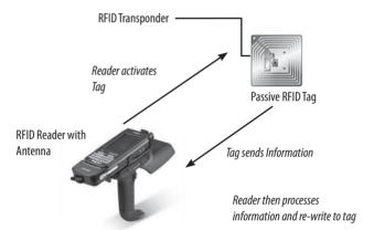
Figure 1: RFID Reader and Tag Communication Flow Diagram Source: Aydın et.al.(2012), p.163
