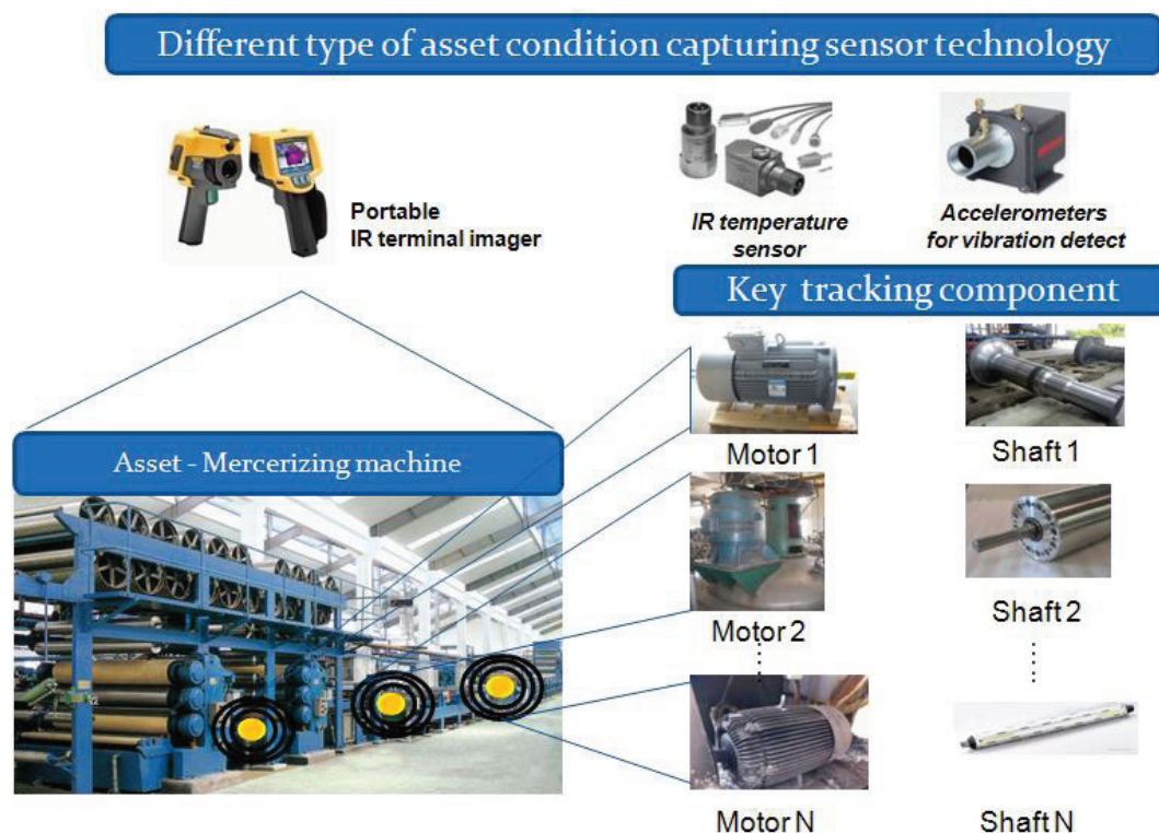
Figure 2: Smart Sensors Used in a Key Asset Component
